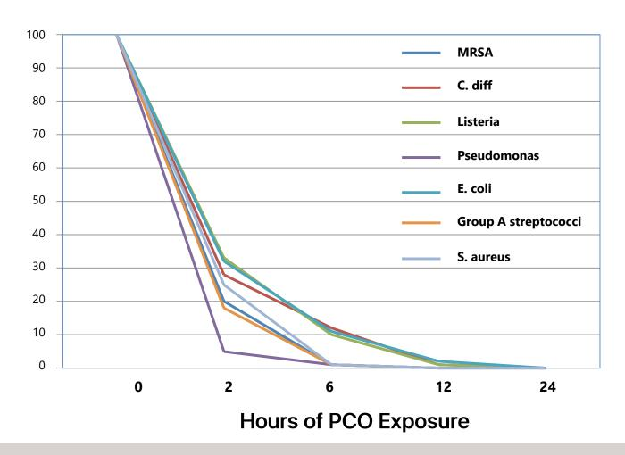
Photocatalytic oxidation used to actively reduce airborne and surface pathogens. Selected microorganism prepared and placed on a stainless-steel surface, allowing analysis at 2 hours, 6 hours, 12 hours, and 24 hours. After 24 hours exposure to PCO, organism's viability was reduced between **96.4% and 99.9%** (3).
