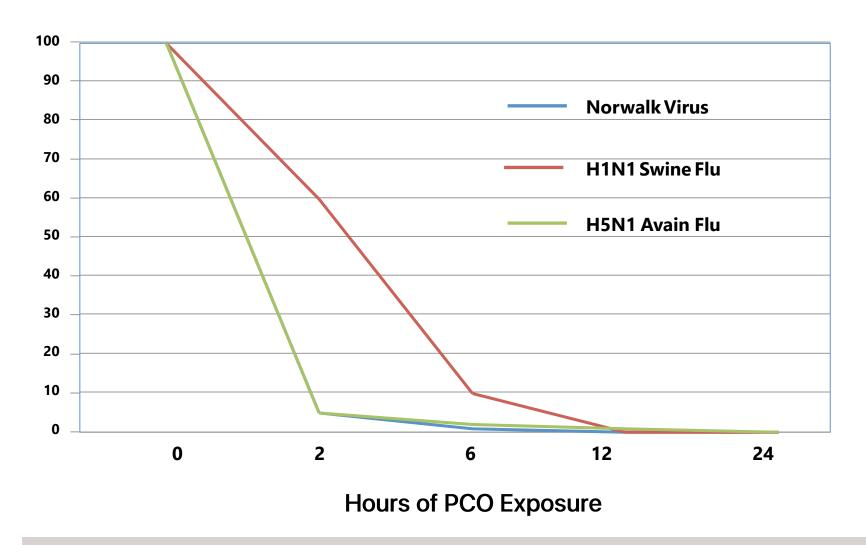
Photocatalytic oxidation on used to actively reduce airborne and surface pathogens. Selected microorganism prepared and placed on a stainless-steel surface, allowing analysis at 2 hours, 6 hours, 12 hours and 24 hours. After 24 hours exposure to PCO, organism's viability was reduced between **96.4% and 99.9%** (11, 13)
